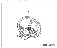
(1) When the button (1) is pressed, the horn will sound.
