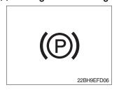
(1) This LED lights when the parking brake is activated.
