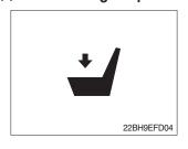
This LED lights when the operator is not on the seat.
