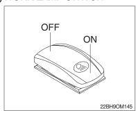
(1) This switch is used to operate work lamps. Press this switch to turn on work lamps.
