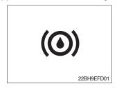
This LED lights when measured level of brake oil stored in reservoir tank is below the minimum acceptable mark.
